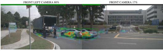
Figure 22: Raw cross-attention examples for objects (green OBB) that lie in the overlapping FOV of two cameras. In each example, a single query is used to generate the saliency maps for all camera images. Attention can be observed on the object on both overlapping camera images. We further approximated the contribution of each camera for a detection by computing the faction of attention for each camera, indicated by the green bar and the percentage data.
